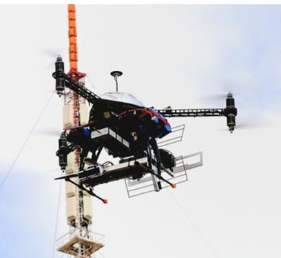
The UAV with the measurement payload
